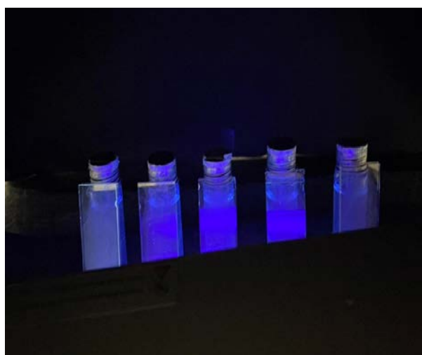
Fig. 1: Methylene blue samples (2 pm, 4 ppm, 6ppm, 8 ppm and 10 ppm) irradiated with UVA-UBV light for several hours and absorbance UV-VIS spectrum from 200 to 700 nm, showing an increasing after light contact in all cases.
