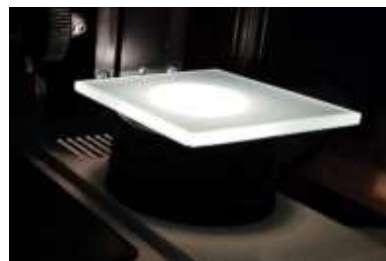
Fig. 1 Solar concentrator deposited with plasmonic nanoparticles
